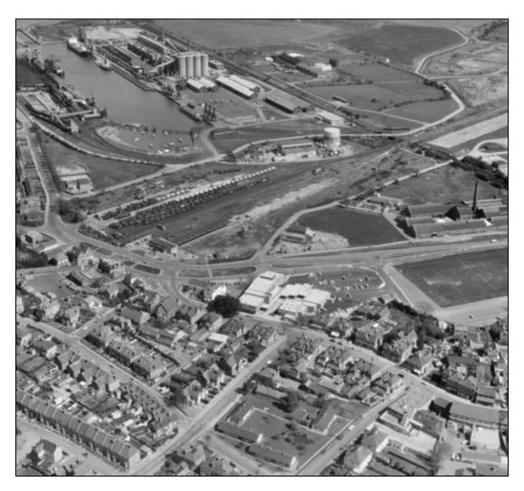
The area of the creek between the railway (still curving across the scene and into the dock area) and the town was entirely reclaimed in the 1920s/1930s by dumping the power station excavation spoil onto the area.
